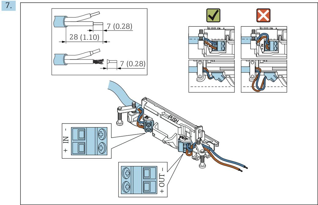
Ensure that the cores are of sufficient length to be connected in the field device. Do not shorten the cores to the required length until you are connecting them in the field device.
