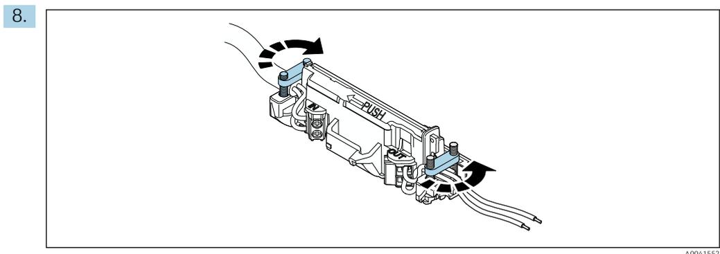
Tighten screws for strain relief. Torque: 0.4 Nm ± 0.04 Nm
