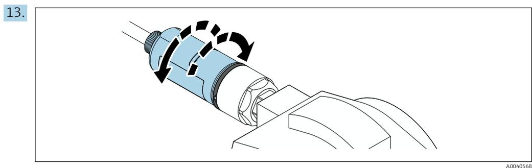
Align the bottom housing section with the transmission window according to the network architecture →
