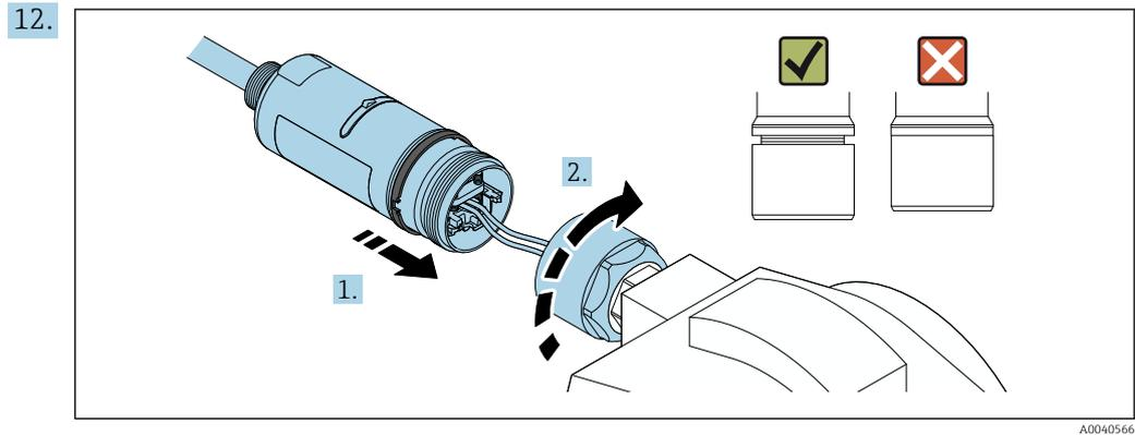
Do not tighten the top housing section yet, so that you are still able to rotate the bottom housing section.
