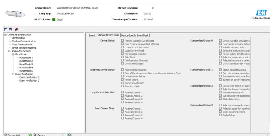
6. Activate the desired event notifications in the "Device-Specific Event Mask" tab. To do so, select the check box in front of the particular event. Multiple notifications can be selected. Observe the Operating Instructions for the selected device in the "Device Index" parameter.
