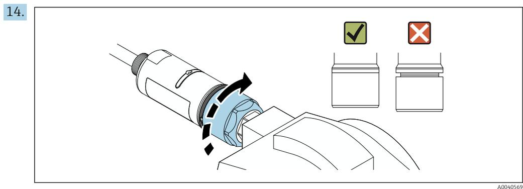
Tighten the top housing section so that the blue design ring can still be rotated afterwards. Torque:  $5 \text{ Nm} \pm 0.05 \text{ Nm}$
