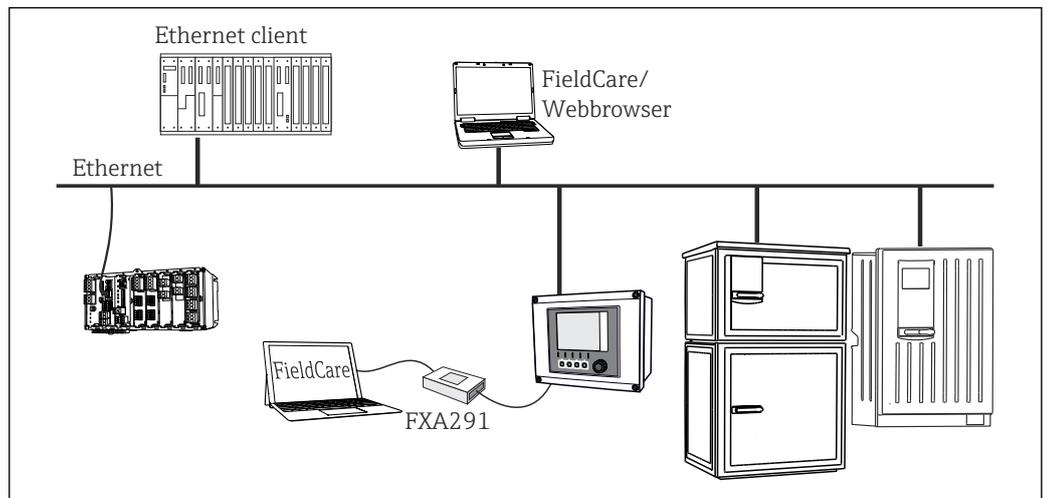
22 Modbus TCP o EtherNet/IP o PROFINET
