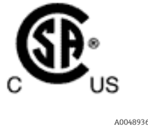
Figure 5. Label showing equipment is approved for use in hazardous areas in the United States and Canada
