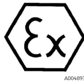
Figure 6. ATEX label for use in hazardous areas
