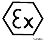
Figure 3. ATEX label for use in hazardous areas
