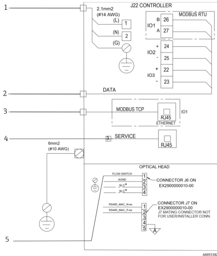
Fig 12. J22 analyzer electrical connections
