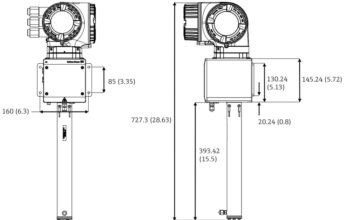
Fig 5. J22 TDLAS Gas Analyzer wall mount (without panel) mounting dimensions, mm (in)
