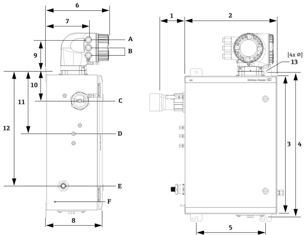
Fig 7. Mounting dimensions, J22 TDLAS Gas Analyzer with enclosed SCS
