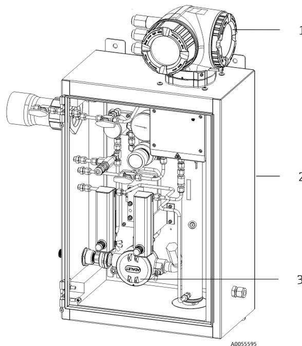
Fig 3. J22 TDLAS gas analyze in an enclosure
