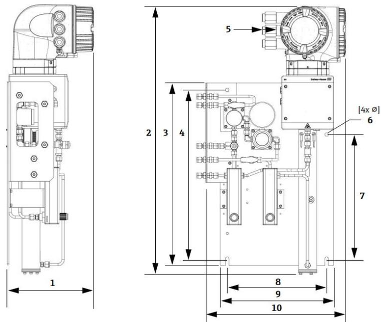
Fig 6. Mounting dimensions, J22 TDLAS Gas Analyzer with SCS on panel
