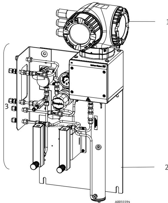
Fig 2. J22 TDLAS gas analyzer on a panel
