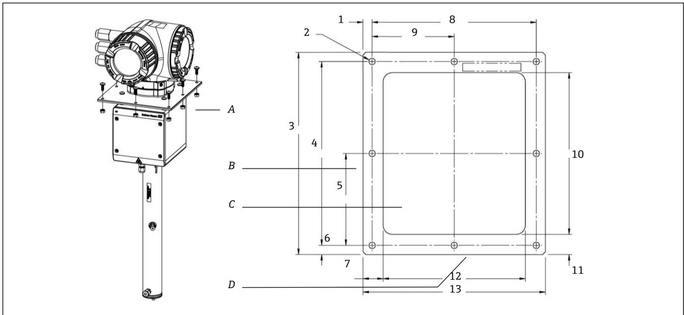
Fig 10. Mounting dimensions, bracket, and hardware for plate-mounted J22 TDLAS Gas Analyzer
