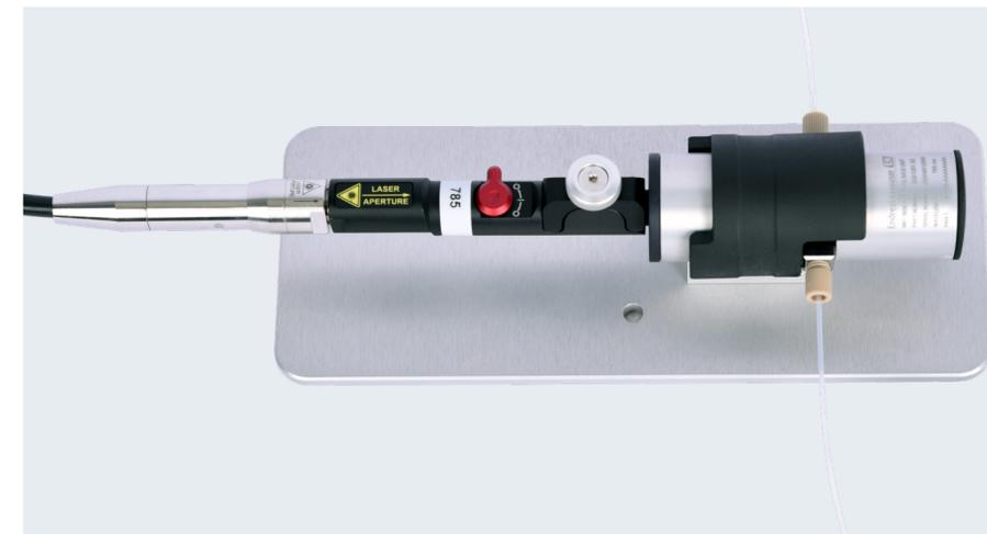
(Top) micro flow cell and flow bench components; (bottom) Raman flow assembly connected to an Rxn-10 probe
