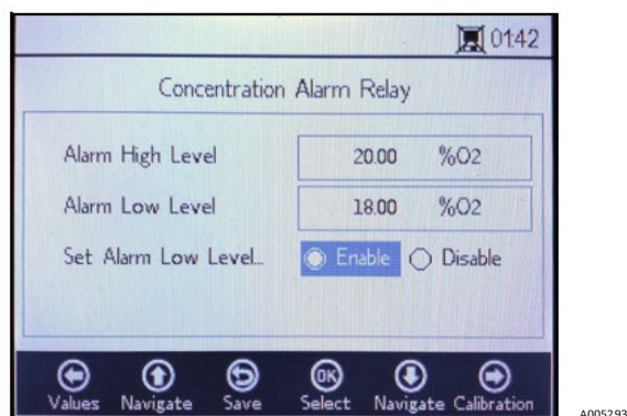
Figure 69. Analogues - Concentration alarm relay
