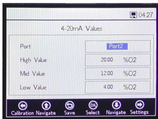
Figure 68. 4-20mA values for mode "Bilinear"
