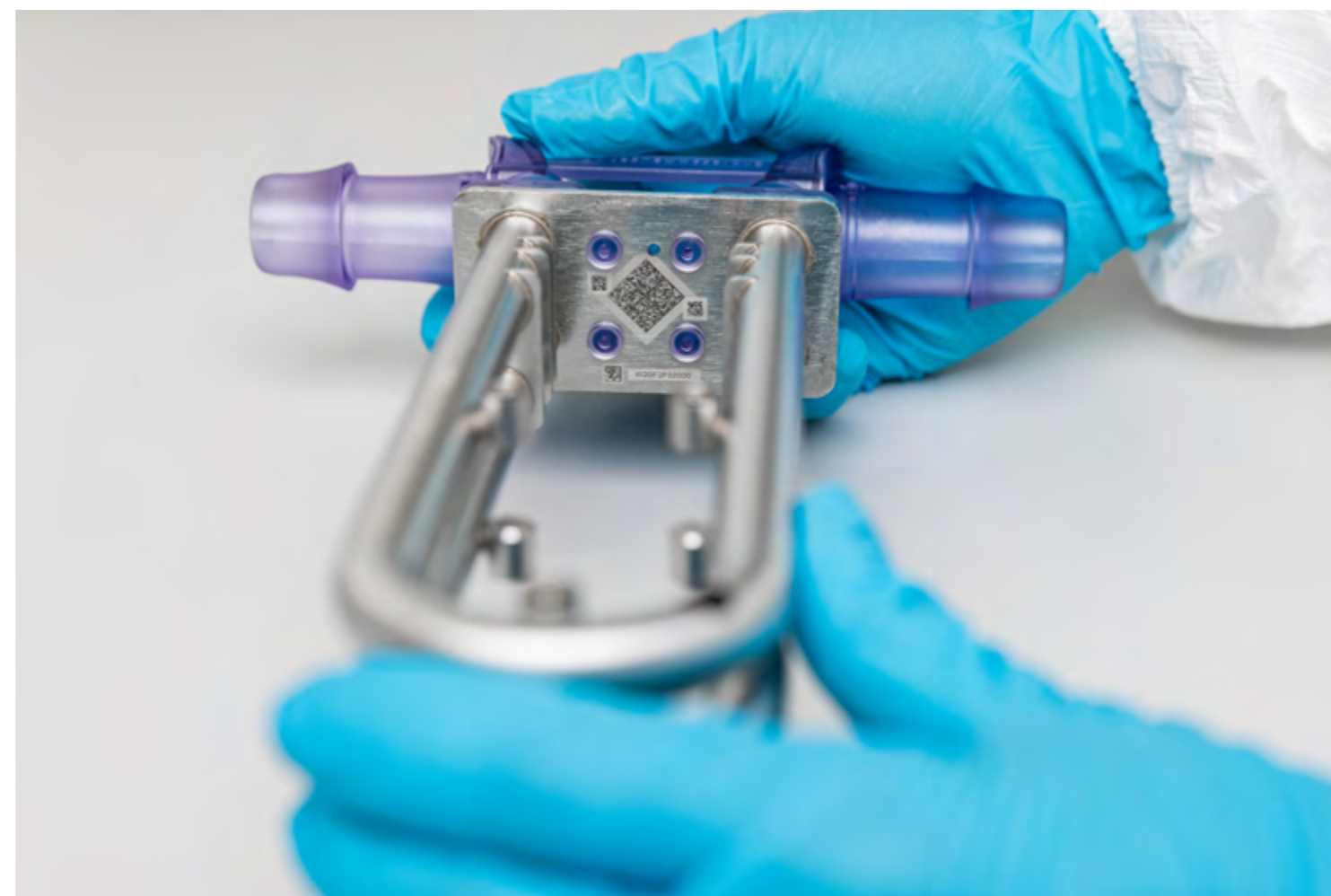
3. The QR code on the disposable part contains the factory calibration data
