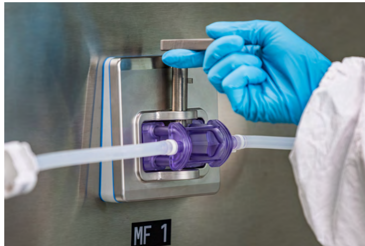
1. The clamping mechanism can be easily opened with one hand
