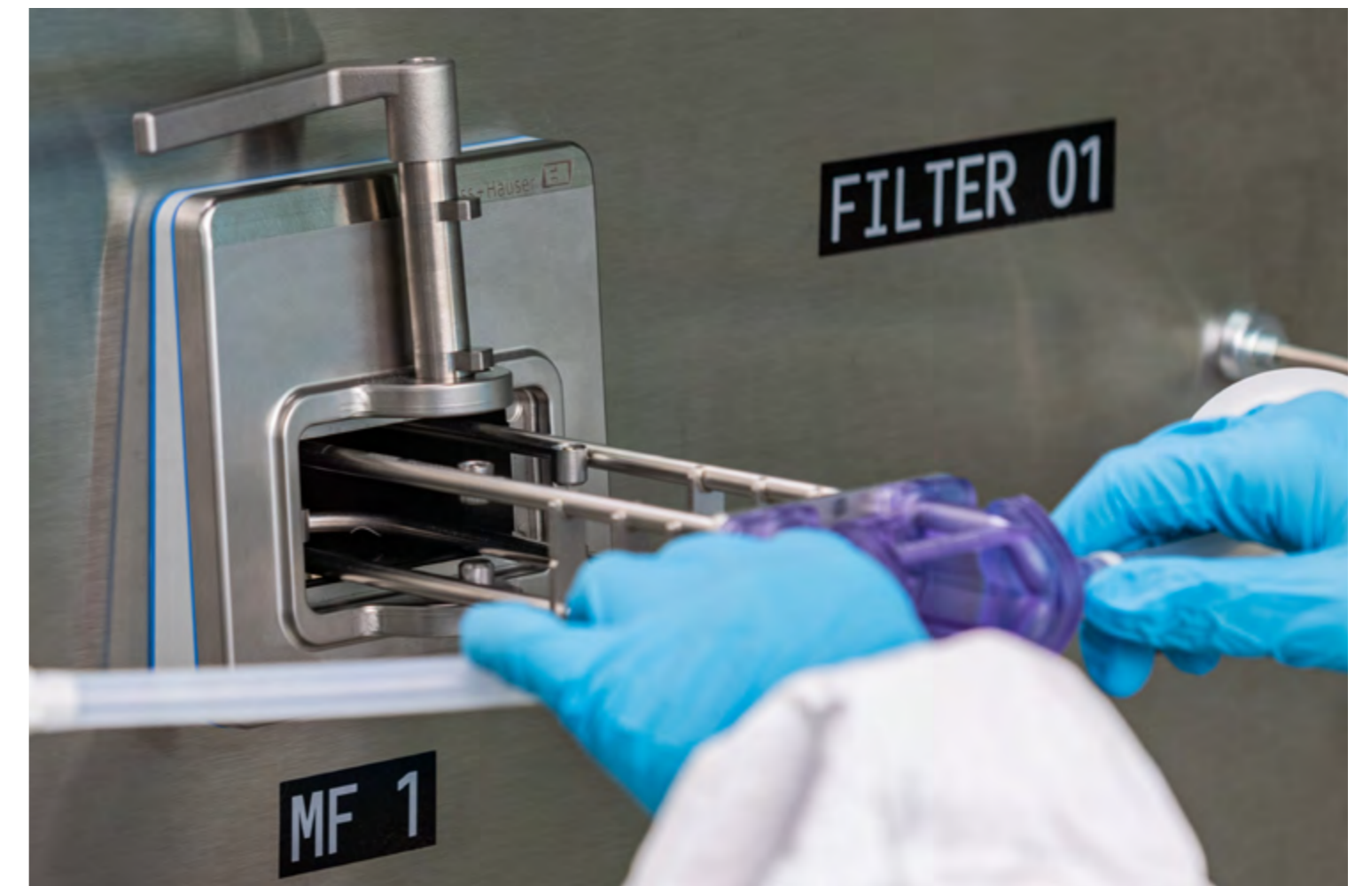
2. The disposable measuring tube can then be removed
