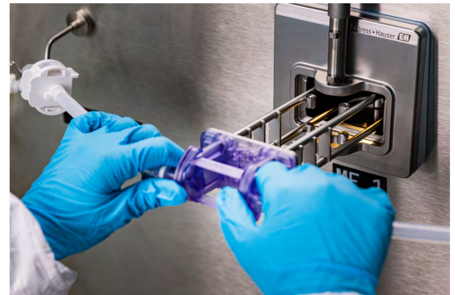
4. The calibration data is read out by the camera in the base unit
