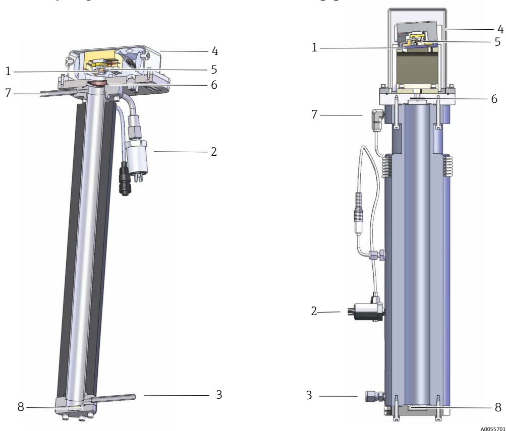
Figure 1: Schematic of a typical laser diode absorption spectrometer:
