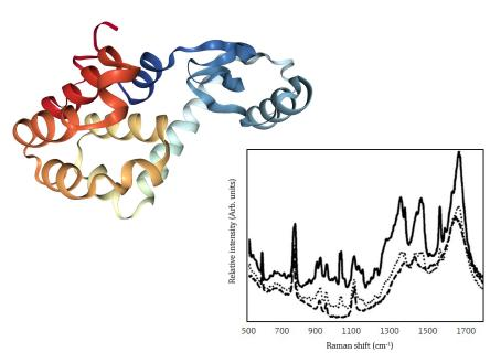
The protein structure of lysozyme (left) is affected by temperature, pH, precipitating agent, and crystallization time.¹ Raman spectra of lysozyme is depicted in the presence of acetate buffer at 90 mg/ml (right, top), 30 mg/ml (right, middle) and 0 mg/ml (right, bottom).
