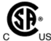
Figure 3. Label showing equipment is approved for use in hazardous areas in the United States and Canada
