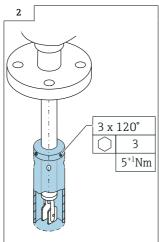
➤ This version is only suitable for pipe extensions. The fork protection must be parallel to the pipe extension. Tighten the screws with the required torque.
