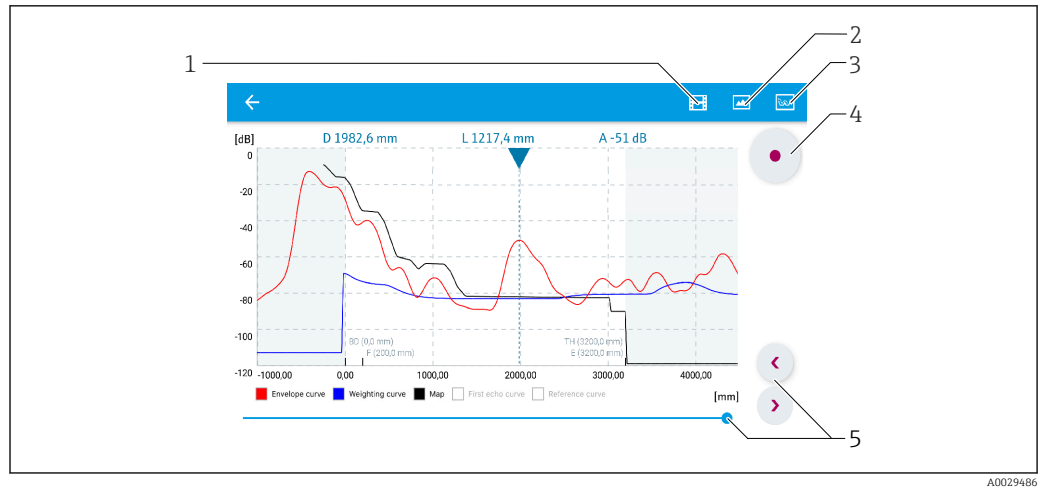
31 Envelope curve display (sample) in SmartBlue for Android
