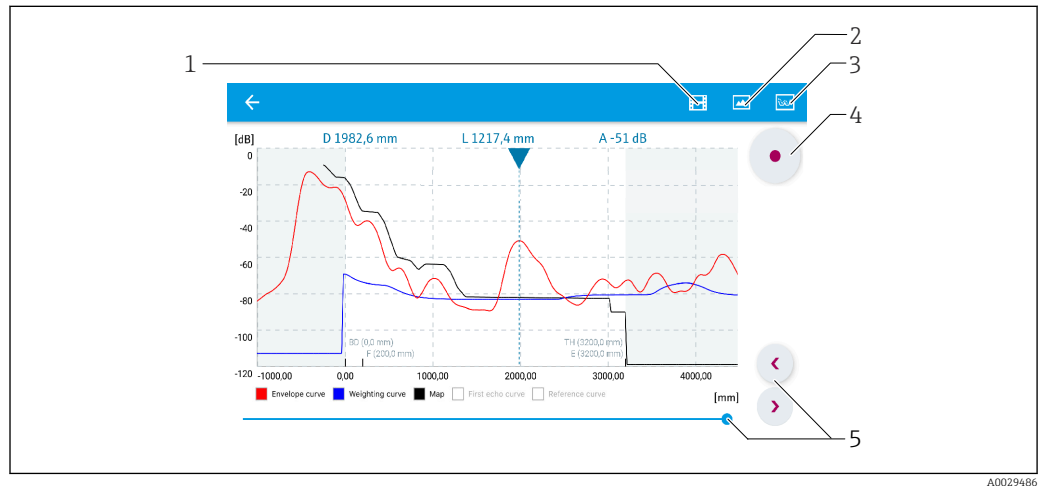
35 Envelope curve display (sample) in SmartBlue for Android
