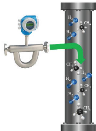
**Figure 6:** Measuring just the volume of hydrogen blended can't determine the final mix ratio.
