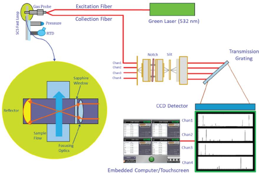
**Figure 5:** The ability to connect a gas probe to the analyzer using fiberoptic cables eliminates the need for sample transport to the analyzer. The probes can be designed to handle samples at or near process pressures and temperatures
