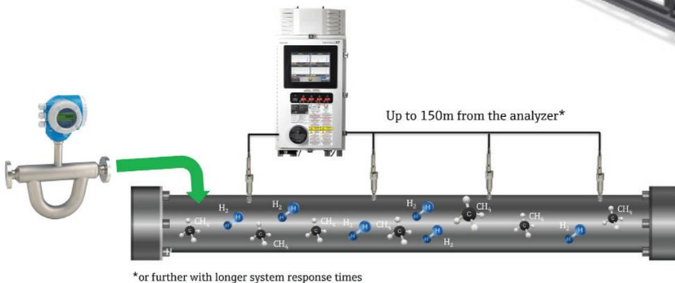
**Figure 8:** Using multiple Raman probes over a long length of pipeline can help determine how hydrogen mixes into the flow after injection.
