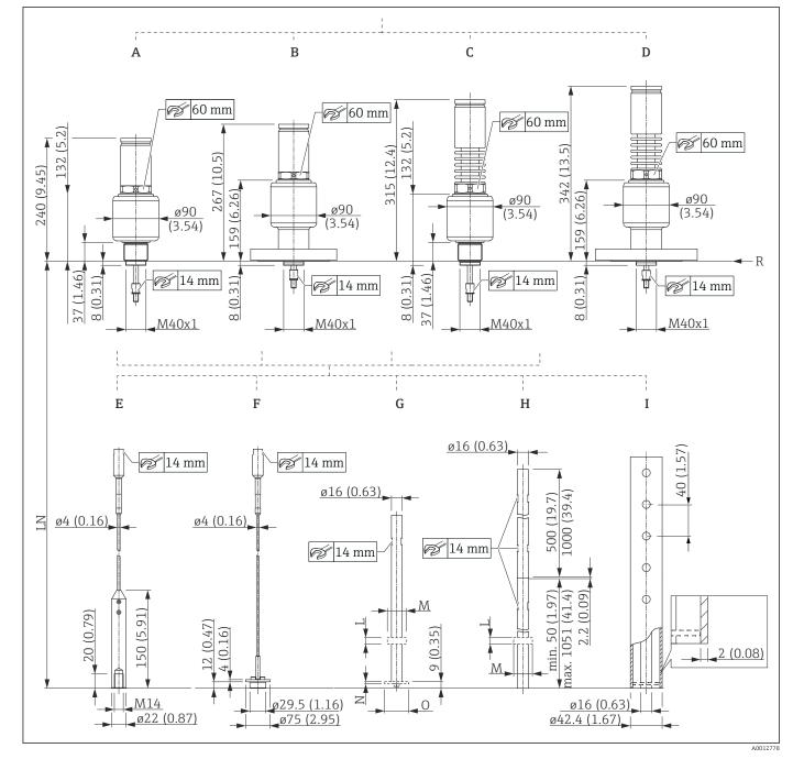
FMP54: Dimensions of process connection/probe
