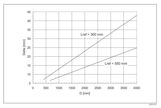
D Distance from lower edge of the flange to product DeltaMeasurement error
