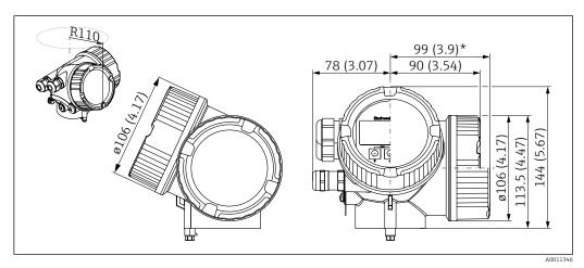
42 GT19 housing (plastic PBT). Unit of measurement mm (in)
