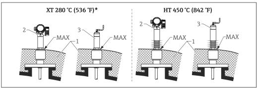
€ 40 Process connection with flange - sensor version XT and HT
