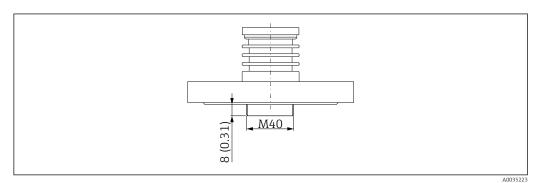
$\blacksquare$  48 Dimensions of AlloyC flanges. Unit of measurement mm (in)
