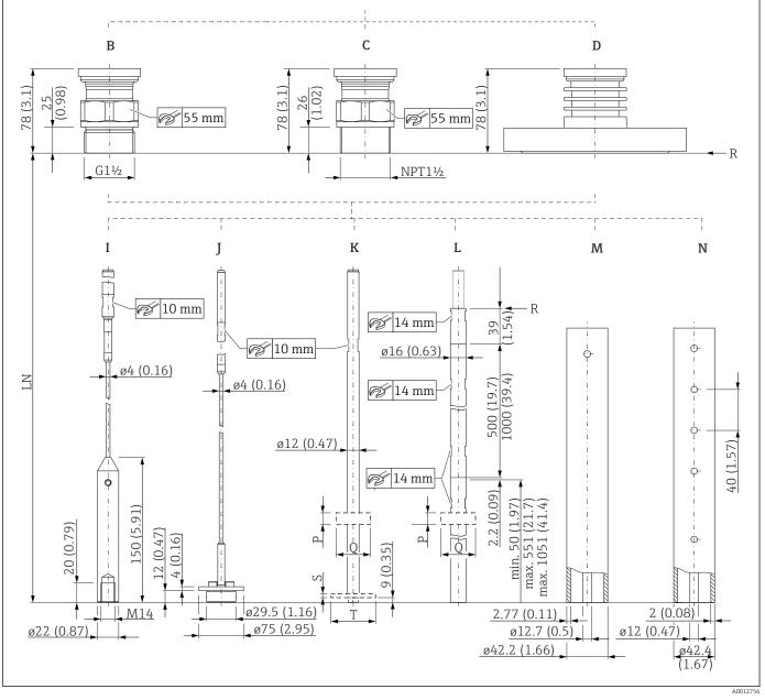
FMP51: Dimensions of process connection (G1½,NPT1½, flange)/probe
