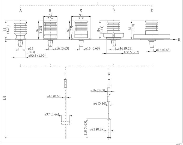
FMP52: Dimensions of process connection/probe
