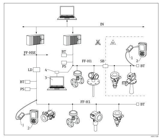
■ 57 FOUNDATION Fieldbus system architecture with associated components
