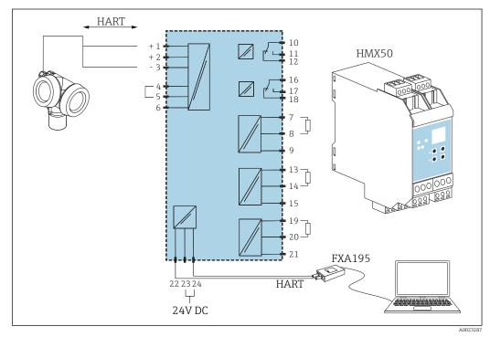
■ 26 Connection diagram for HART loop converter HMX50 (example: passive 2-wire device and current outputs connected as power source)
