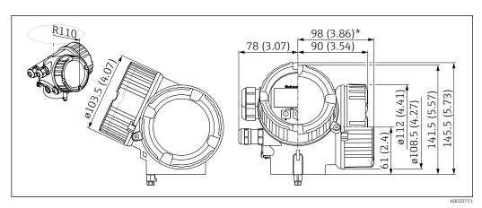
■ 43 Housing GT20 (aluminum coated). Unit of measurement mm (in)
