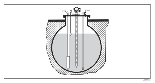
In the case of nozzles with large diameters, use a coaxial probe to avoid reflections at the nozzle wall.
