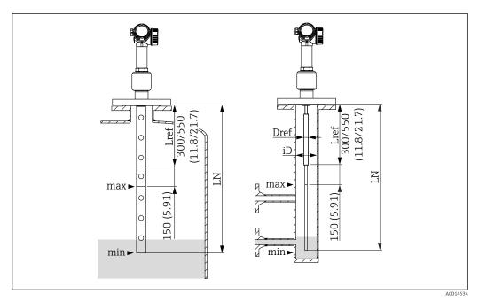
■ 33 FMP54 with reference signal for gas phase compensation; unit: mm (in)
