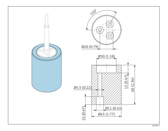
The centering weight is suitable for probes with a rope diameter of 4 mm ( $\frac{1}{6}$  in) and can be used in DN50/2" pipes.
