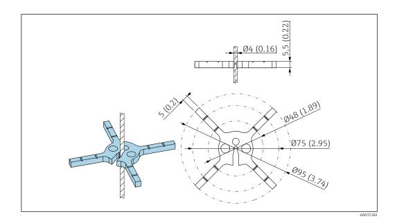
The centering star is suitable for probes with a rope diameter of 4 mm ( $\frac{1}{6}$  in) (including coated rope probes).
