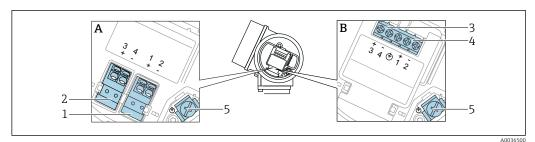
Terminal assignment, 2-wire: 4 to 20 mA HART, 4 to 20 mA
