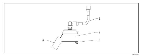
Materials: Adapter and cable for "Remote sensor" version
