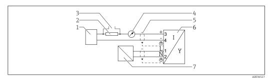
$\blacksquare$  23 Function diagram 4-wire: 4 to 20 mA HART (90 to 253  $V_{AC}$ )
