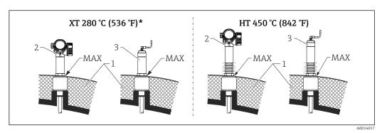
Process connection with thread - sensor version XT and HT
