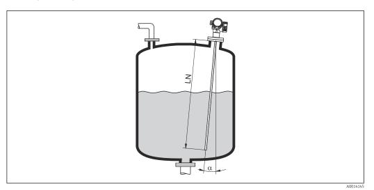
• For mechanical reasons, the probe should be installed as vertically as possible.
