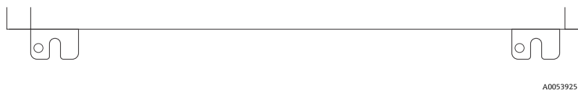
Figure 7. Slotted bottom mounting tabs of enclosure
