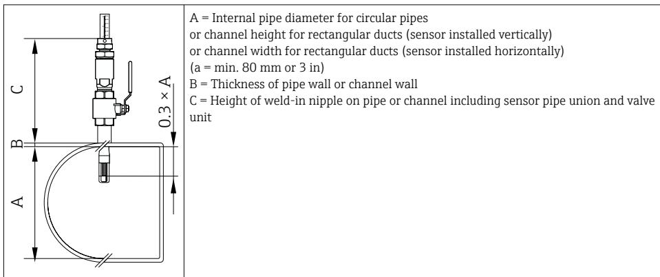
Determining the insertion depth for t-mass B 150, I 300, 500-digital:
