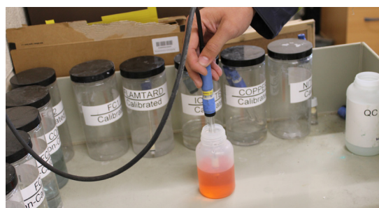
Convenient offline calibration is possible with Memosens
