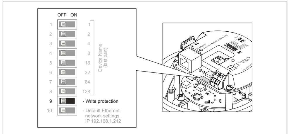
Setting the write protection switch on the main electronics module to the **On** position enables hardware write protection. Setting the write protection switch on the main electronics module to the **Off** position (factory setting) disables hardware write protection.
