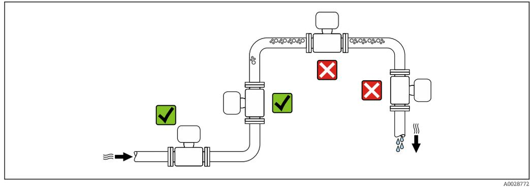
To prevent measuring errors arising from accumulation of gas bubbles in the measuring pipe, avoid the following mounting locations in the piping:
