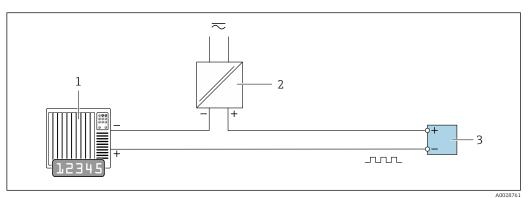
16 Connection example for pulse/frequency output (passive)
