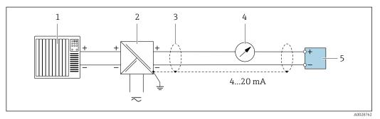
12 Connection example for 4 to 20 mA HART current output (passive)
