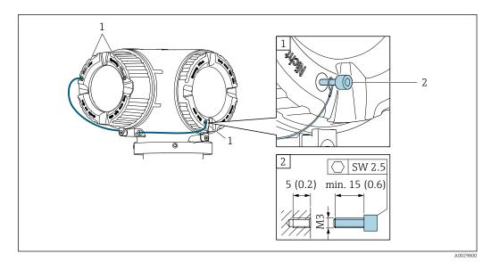
*1 Cover borehole for the securing screw*
