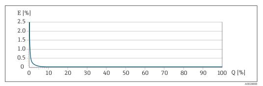
*E Maximum measurement error in % o.r. (example with PremiumCal)*
