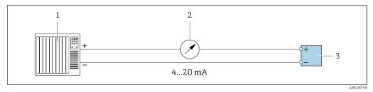
I4 Connection example for 4-20 mA current output (active)
