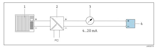
■ 15 Connection example for 4-20 mA current output (passive)
