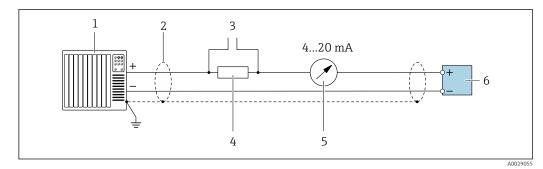
🖸 11 Connection example for 4 to 20 mA HART current output (active)
