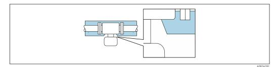
6 Thermal insulation with exposed extended neck
