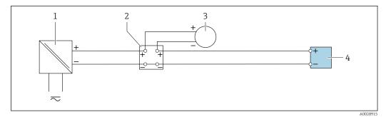
■ 21 Connection example for 4 to 20 mA current input
