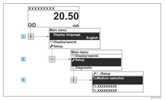
31 Navigation to "Setup" menu using the example of the local display
