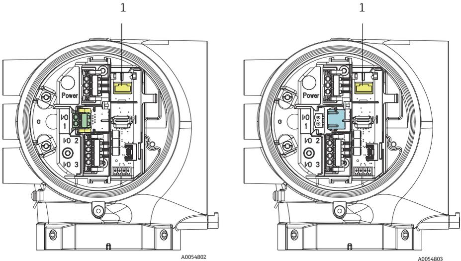
Figure 22. Service interface CDI-RJ45 (1) connections for I/O1 with Modbus RTU/RS485/2-wire (left) and Modbus TCP/Ethernet/RJ45 (right)
