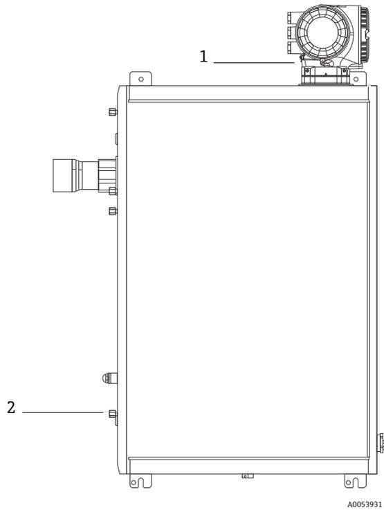
Figure 9. Ground connections
