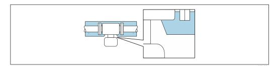
8 Thermal insulation with exposed extended neck
