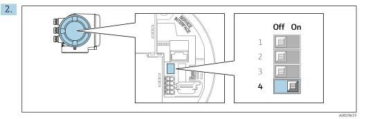
To switch addressing from software addressing to hardware addressing: set the DIP switch to  $\mathbf{On}.$
