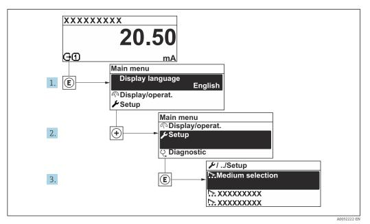
36 Navigation to "Setup" menu using the example of the local display
