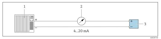
☑ 19 Connection example for 4-20 mA current output (active)
