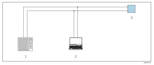
■ 32 Options for remote operation via Modbus RS485 protocol (active)
