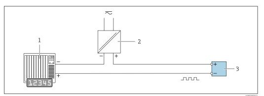
21 Connection example for pulse/frequency output (passive)
