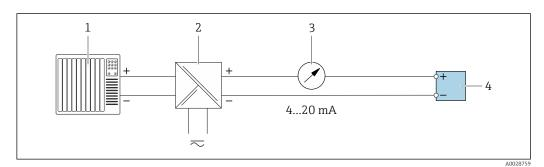
■ 20 Connection example for 4-20 mA current output (passive)
