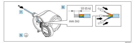
7. Push the cable through the cable entry. To ensure tight sealing, do not remove the sealing ring from the cable entry.
