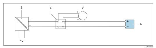
🛃 26 Connection example for 4 to 20 mA current input
