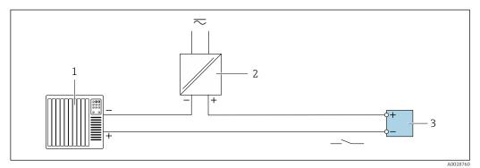
🖻 25 Connection example for relay output (passive)
