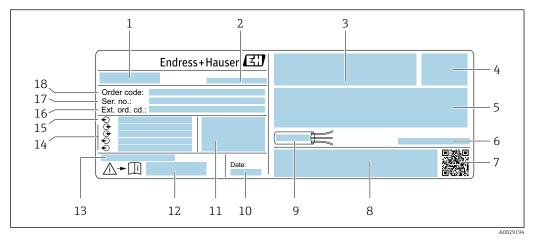
☑ 3 Example of a transmitter nameplate
