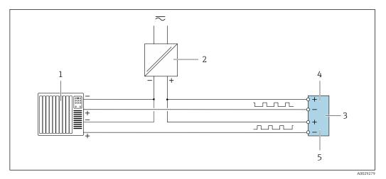
🛃 24 Connection example for double pulse output (passive)
