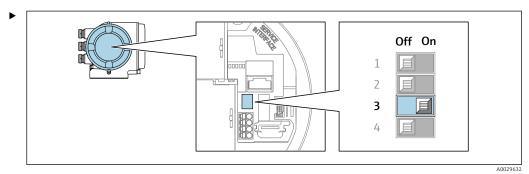
Switch DIP switch no. 3 to **On**.
