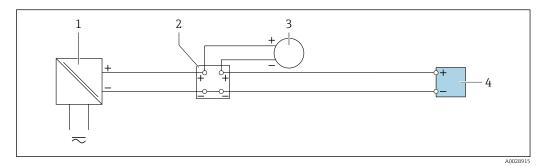
■ 26 Connection example for 4 to 20 mA current input
