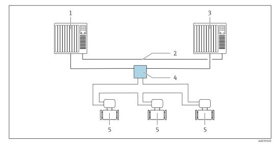
■ 36 Example of the layout of a redundant system (S2): ring topology
