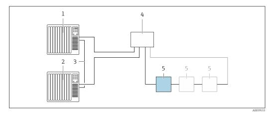
■ 20 Connection example for system redundancy S2
