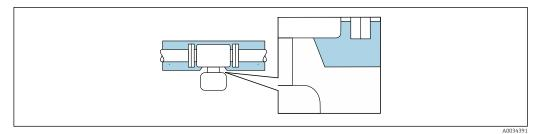
■ 8 Thermal insulation with exposed extended neck
