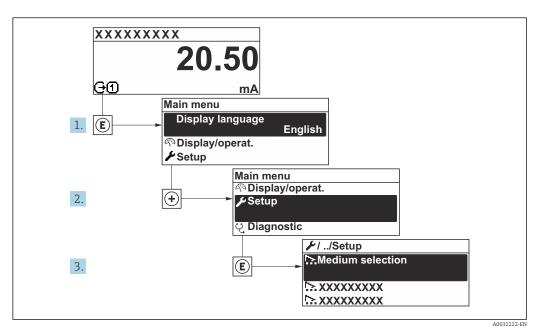
Navigation to "Setup" menu using the example of the local display
