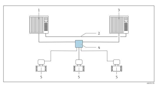
■ 37 Example of the layout of a redundant system (S2): star topology
