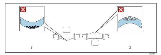
$\blacksquare$  7 Orientation of sensor with curved measuring tube
