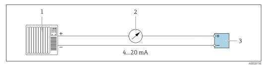
■ 21 Connection example for 4-20 mA current output (active)
