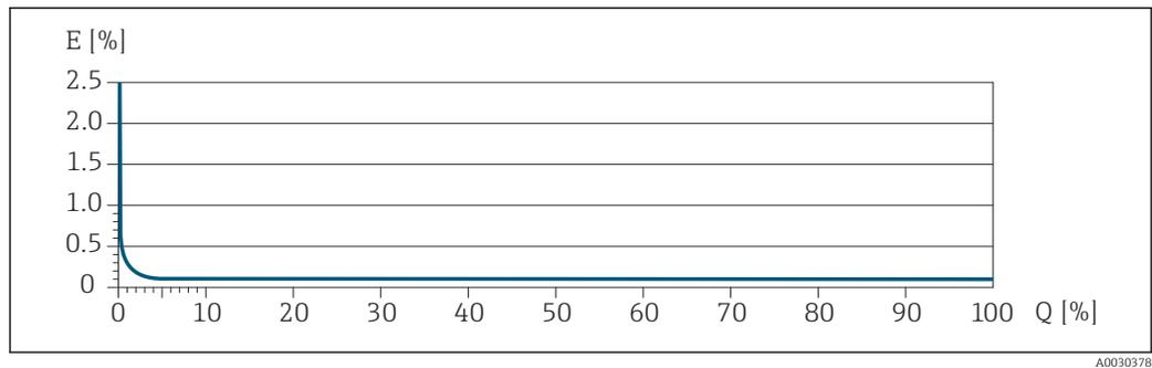
E Maximum measurement error in % o.r. (example)
