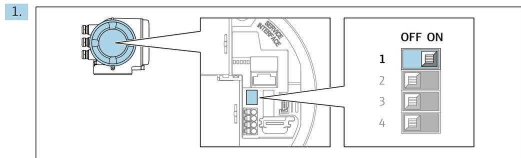
Setting the write protection (WP) switch on the main electronics module to the **ON** position enables hardware write protection.
