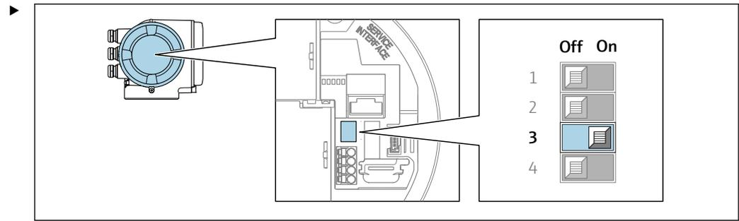
Switch DIP switch no. 3 to **On**.
