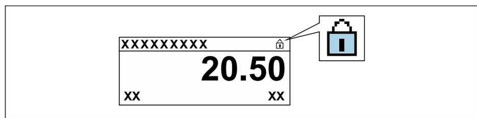
2. Setting the write protection (WP) switch on the main electronics module to the **OFF** position (factory setting) disables hardware write protection.
