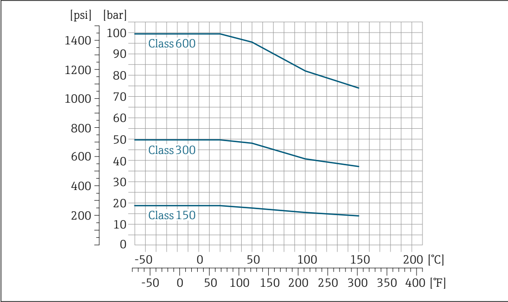
23 With flange material 1.4301 (304); wetted parts: titanium
