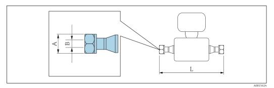
Length tolerance for dimension L in mm: +1.5 / -2.0
