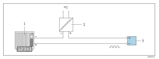
■ 16 Connection example for pulse/frequency output (passive)
