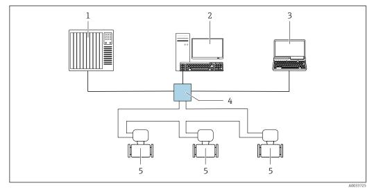
**№** 59 Options for remote operation via EtherNet/IP network: ring topology
