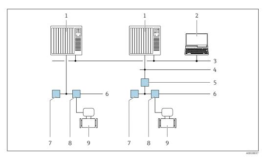
■ 54 Options for remote operation via FOUNDATION Fieldbus network
