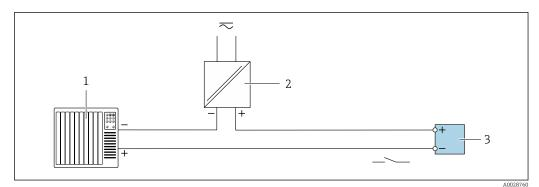
$\blacksquare$  20 Connection example for relay output (passive)
