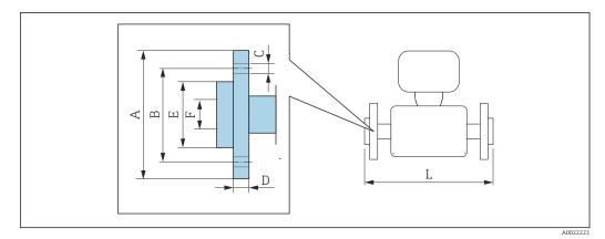
Length tolerance for dimension L in mm: +1.5 / -2.0
