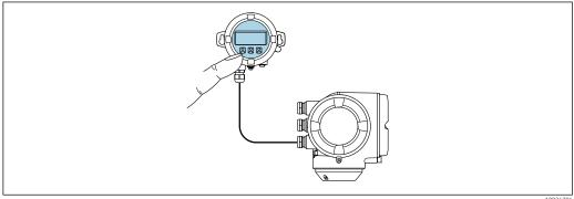
$\blacksquare$  51 Operation via remote display and operating module DKX001
