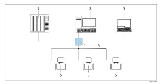
₹ 58 Options for remote operation via EtherNet/IP network: star topology
