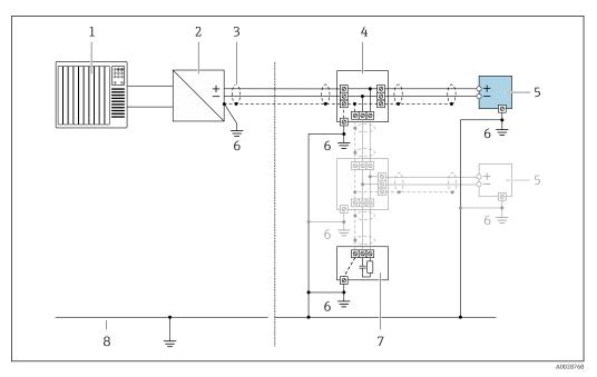
Connection example for FOUNDATION Fieldbus **■** 11
