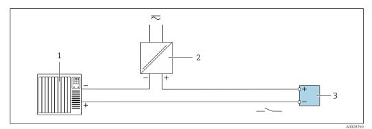
Connection example for switch output (passive)
