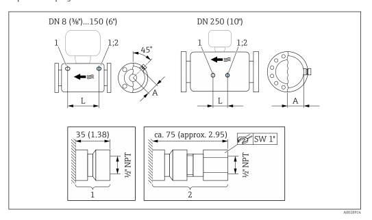
Connection nipple for purge connections: order code for "Sensor options", option CH "Purge connection" Connection nipple with rupture disk: order code for "Sensor option", option CA "Rupture disk"
