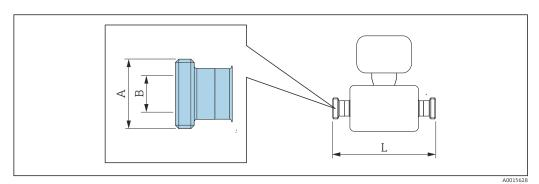
Length tolerance for dimension L in mm: +1.5 / -2.0
