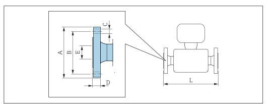
Length tolerance for dimension L in inches: • DN  $\leq$  4": +0.06/-0.08 • DN  $\geq$  6":  $\pm$ 0.14
