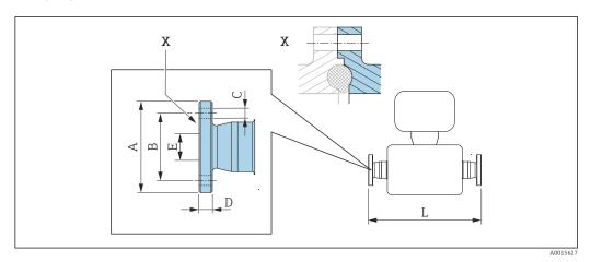
$\blacksquare$  39 Detail X: Asymmetrical process connection; the part shown in blue is provided by the supplier.
