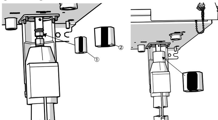
① Insulation tube 20 x 10 mm (Part No. 5325093)
