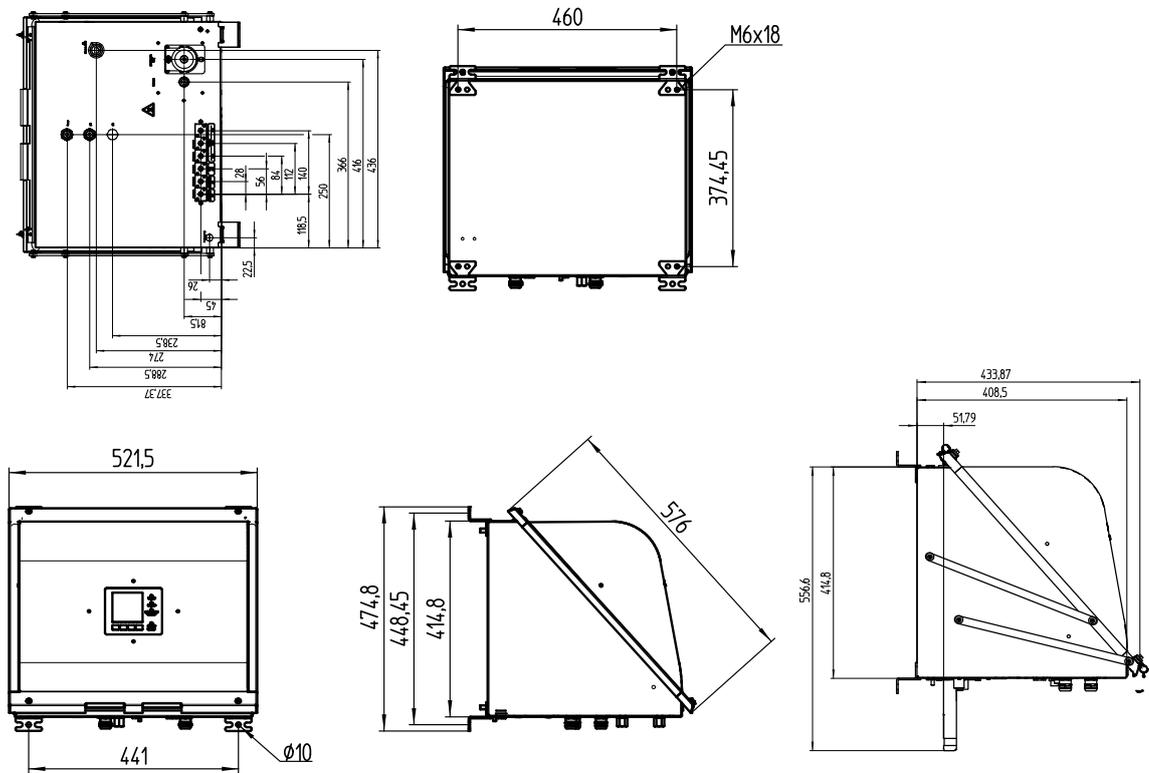
The enclosure is only suitable for attachment on a wall.
