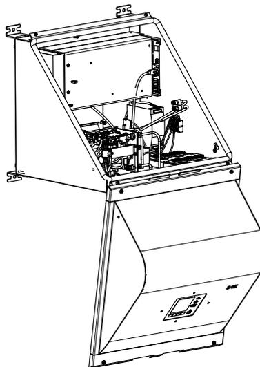
Fig. 63: Flipped cover (opening upwards)
