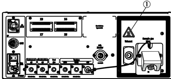
Fig. 2: Warning information on device GMS840 FIDOR
