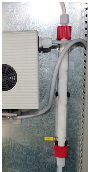
Figure 24: Sample gas fine filter (system-specific)
