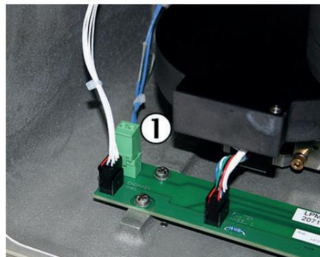
Figure 61: Plug on IR source circuit board
