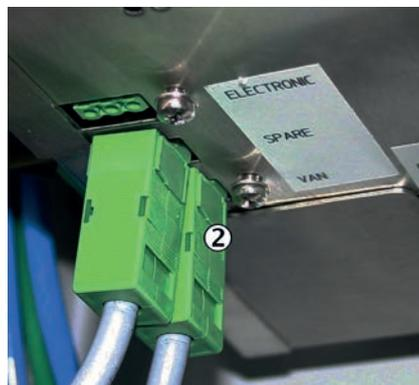
Figure 76: Housing fan plug
