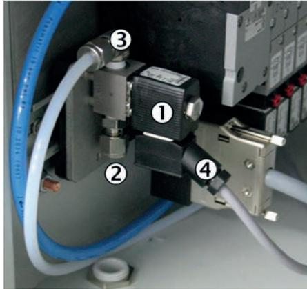
Figure 78: Span gas valve
