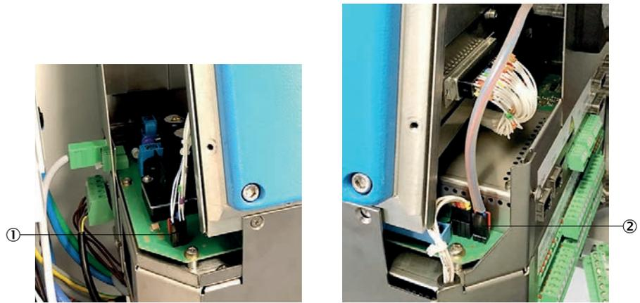
Figure 100: Pressure control module and fan lines
