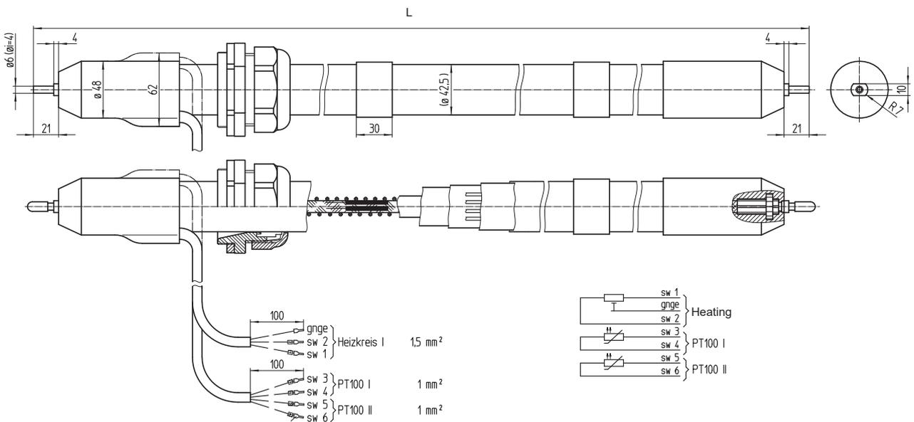
Figure 119: Heated sample gas line
