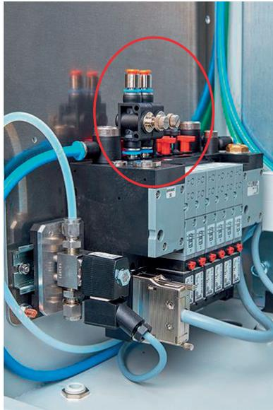
Figure 79: Needle valve on valve block
