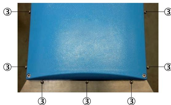
Figure 97: Fastening screws
