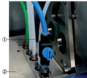
Figure 87: Pressure control module tubes
