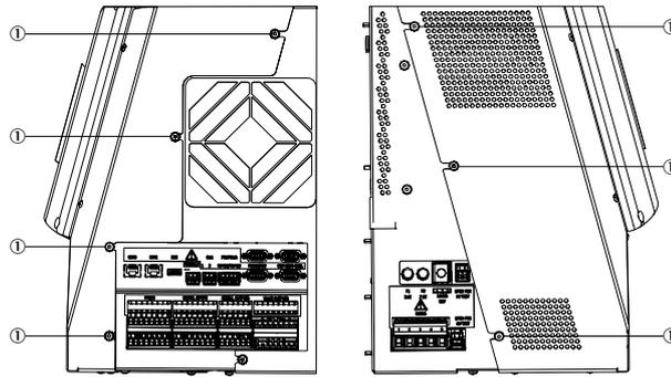
Figure 89: Fastening screws
