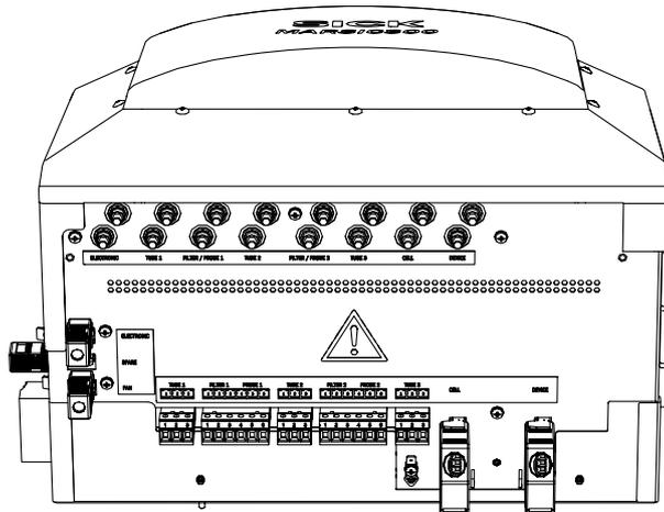
Figure 103: Connections, underside
