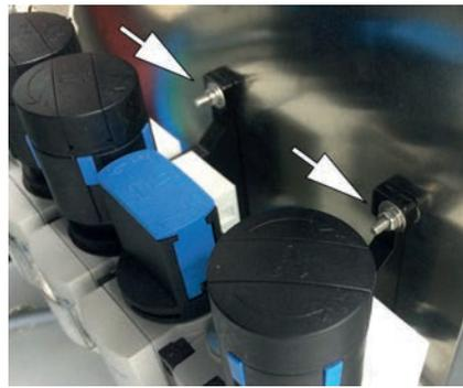
2 top nuts on pressure reducer unit
