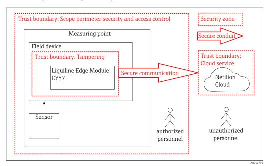
The system structures and system boundaries (trust zones) necessary for the safety consideration differ depending on whether communication with the Netilion cloud platform is via Ethernet or cellular radio.
