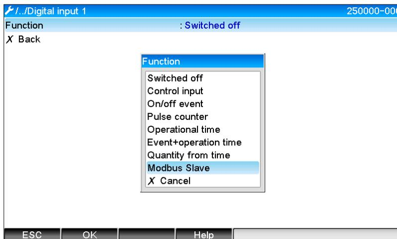
Fig. 5: Setting the digital channel to Modbus
