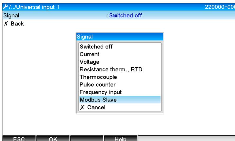
Fig. 4: Setting the universal input to Modbus
