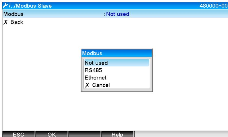
Fig. 2: Selecting the interface for Modbus
