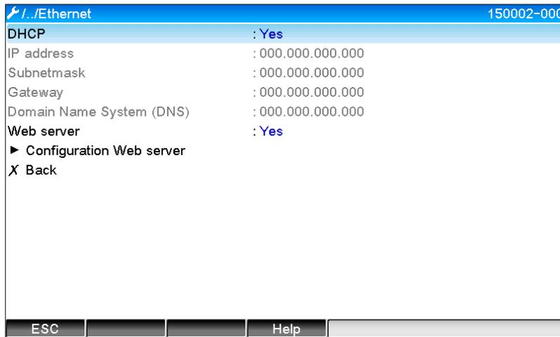
Fig. 3: Settings for the Ethernet interface
