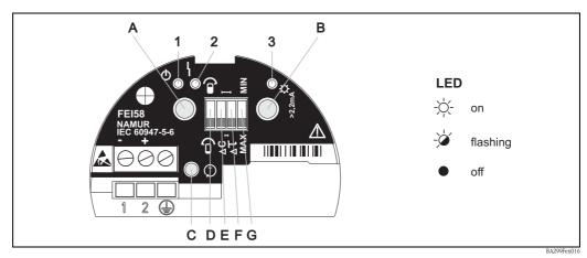
Green LED 1 (♥ ready for operation), red LED 2 ( \ error indicated), yellow LED 3 (★ switching state)
