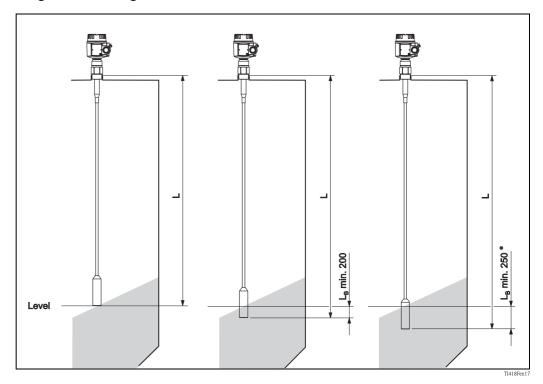
Electrically conductive bulk solids (e.g. coal)
