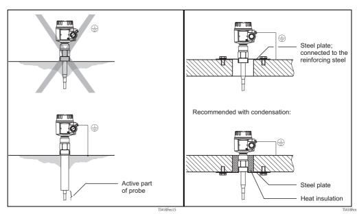
Silo with walls that conduct electricity
