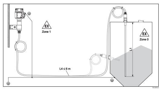
Rod length L1 max.  $4\,\mathrm{m}$ Rope length L1 max.  $19.7\,\mathrm{m}$  (the maximum total length of L1 + L4 should not exceed  $20\,\mathrm{m}$ .)
