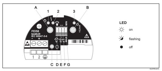
Green LED 1 (♠ operational status), red LED 2 ( ┗ fault message), yellow LED 3 (★ switching status)
