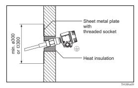
In a silo with concrete walls
