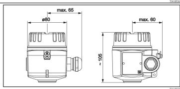
*Aluminum housing F13* with gas-tight process seal
