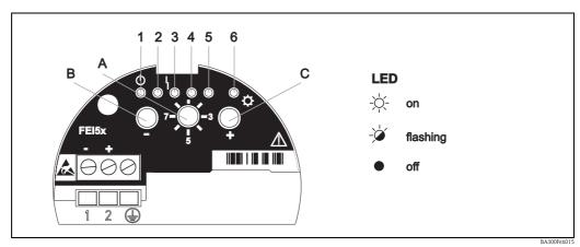
Green LED 1 ( $\bullet$  ready for operation), red LED 3 ( $^{\backprime}$  error indicated), yellow LED 6 (\* switching state)
