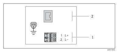
*EtherNet/IP terminal assignment*
