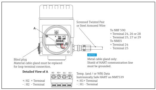
Figure 2: Description of Terminal Board
