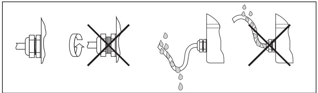
Fig. 8: Connection instructions to retain IP67 protection
