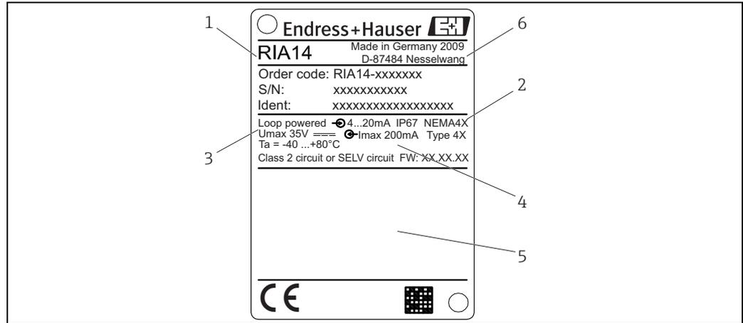
Fig. 1: Nameplate of the field indicator (example)
