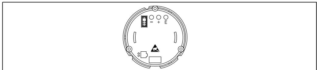
Fig. 10: Operating keys of field indicator ('F', '+', 'E')
