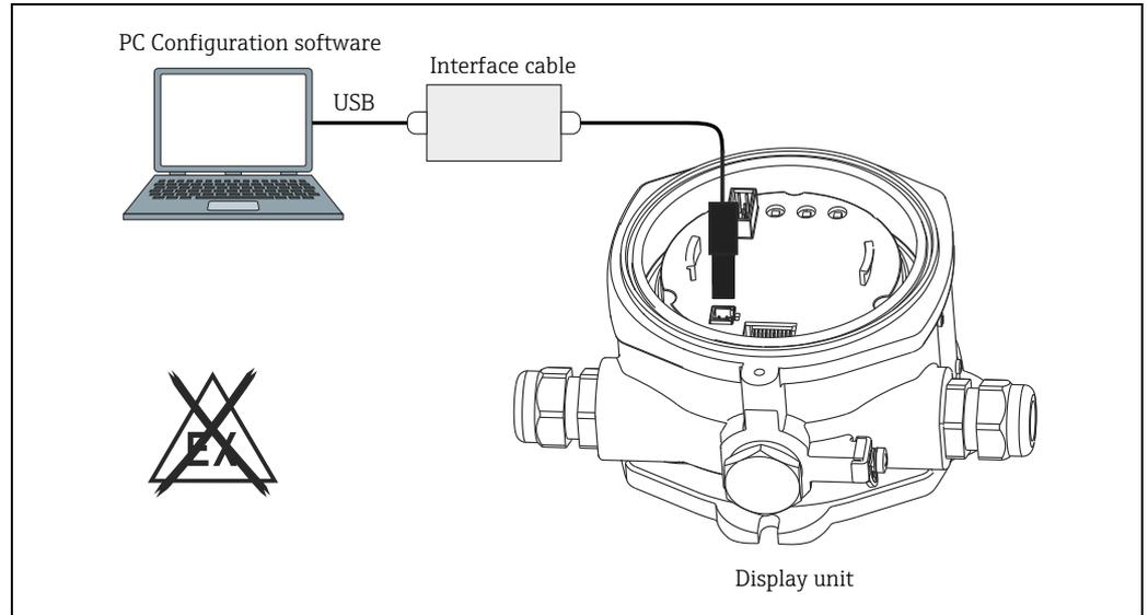
Fig. 17: Configuration with PC operating software.
