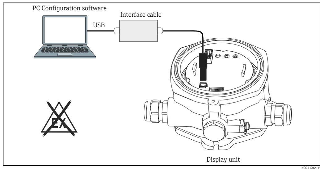
Fig. 12: Configuring the field indicator via interface adapter
