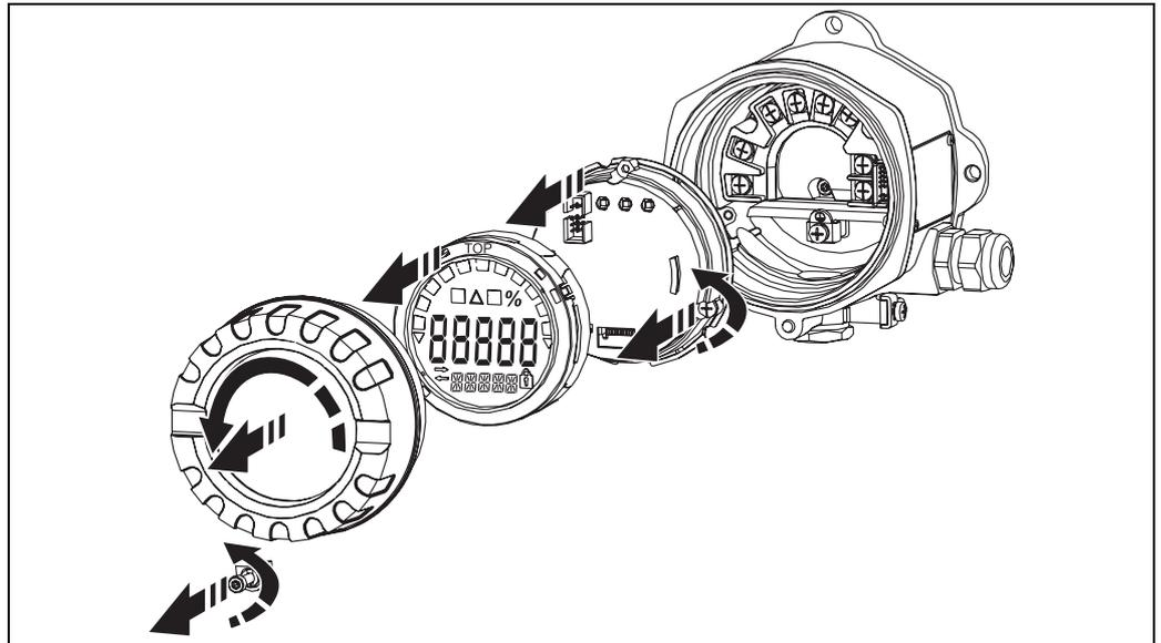
Fig. 6: Opening the housing of the field indicator
