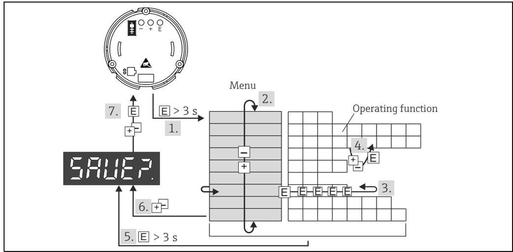
Fig. 11: Programming the field indicator
