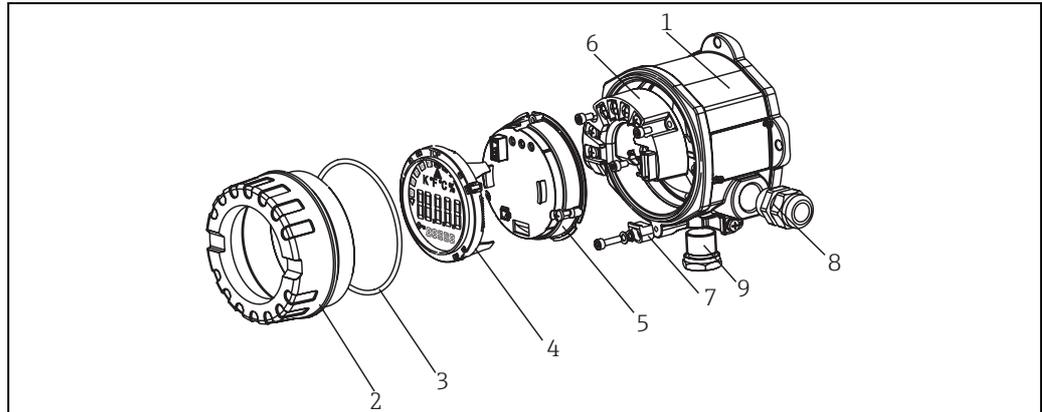
Fig. 14: Spare parts of the field indicator
