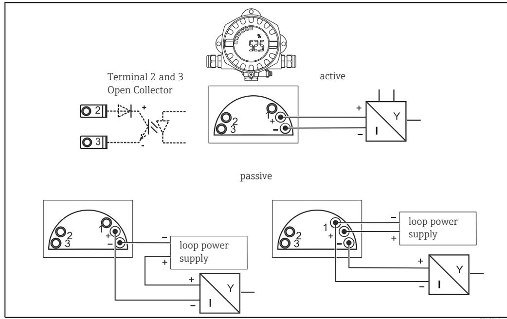
Fig. 7: Terminal assignment
