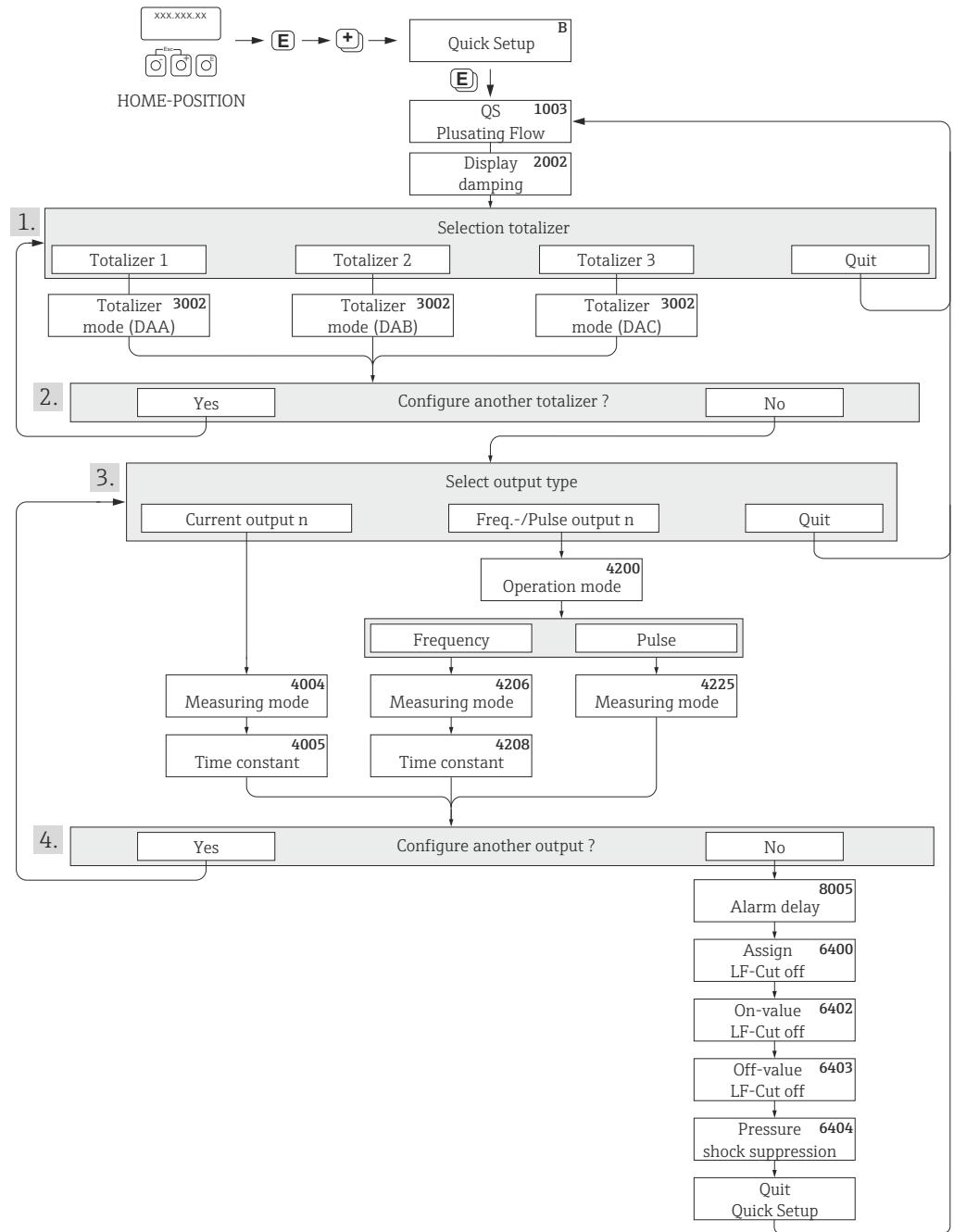
Fig. 6: "QUICK SETUP PULSATING FLOW" menu for operation with severely pulsating flow.
