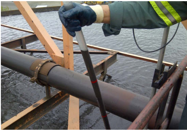
Manual measurement using the "sludge judge".
