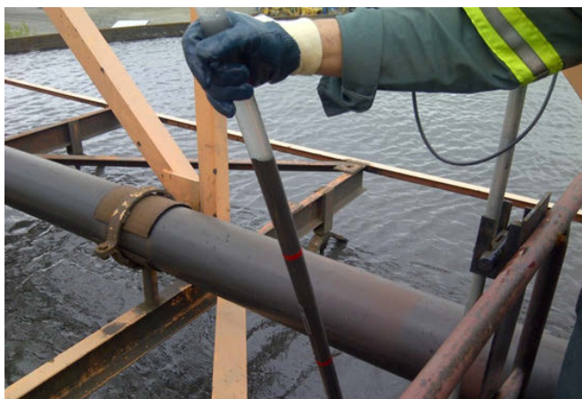
Manual measurement using the "sludge judge".
