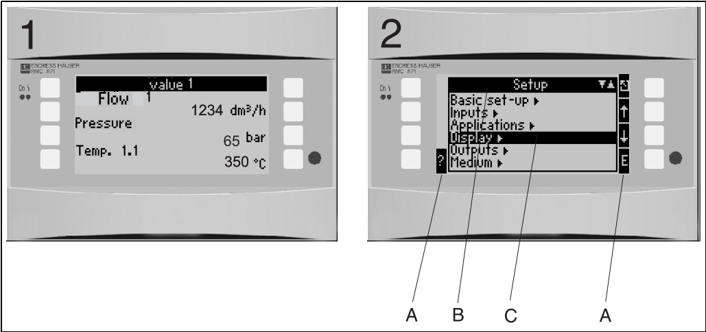
Fig. 16: How the display of the energy computer appears Item: 1: measured value display Item: 2: display of configuration menu item - A: row of key icons - B: current configuration menu - C: configuration menu activated for selection (highlighted in black).
