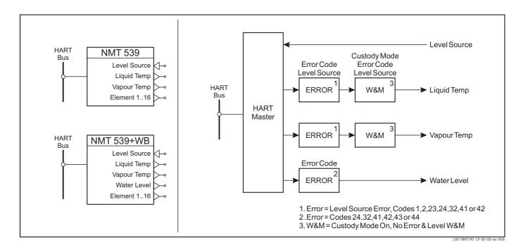
The NMT menu is used for the following types of Endress+Hauser Sakura gauges:
