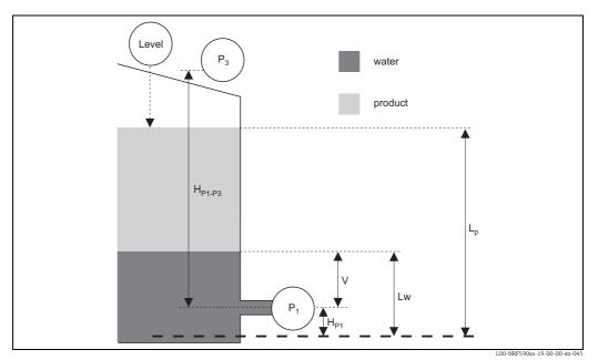
Fig. 6: Principle of HTMS Calculations
