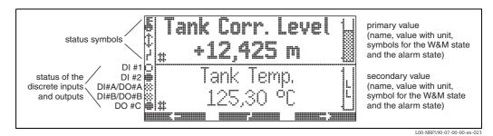
The primary measurement value is constantly displayed in user configured units an format; the secondary value can display up to four alternately measurement values, in a scroll rate choosen by the user.
