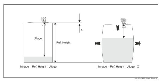
Fig. 8: Hydrostatic tank deformation
