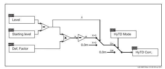
Fig. 10: HyTD Calculation diagram
