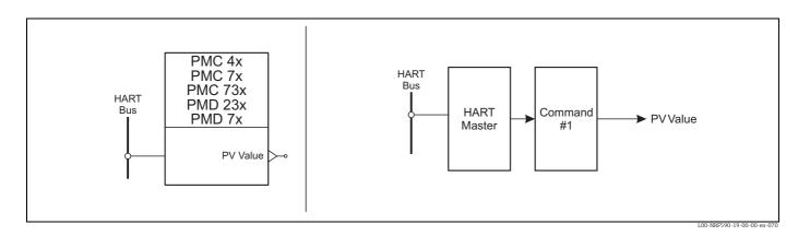
The PMC/PMD menu is used for the following types of Endress+Hauser pressure gauges:
