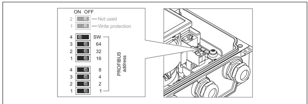
**17** Addressing using DIP switches on the I/O electronics module
