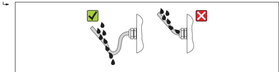
5. Insert dummy plugs into unused cable entries.
