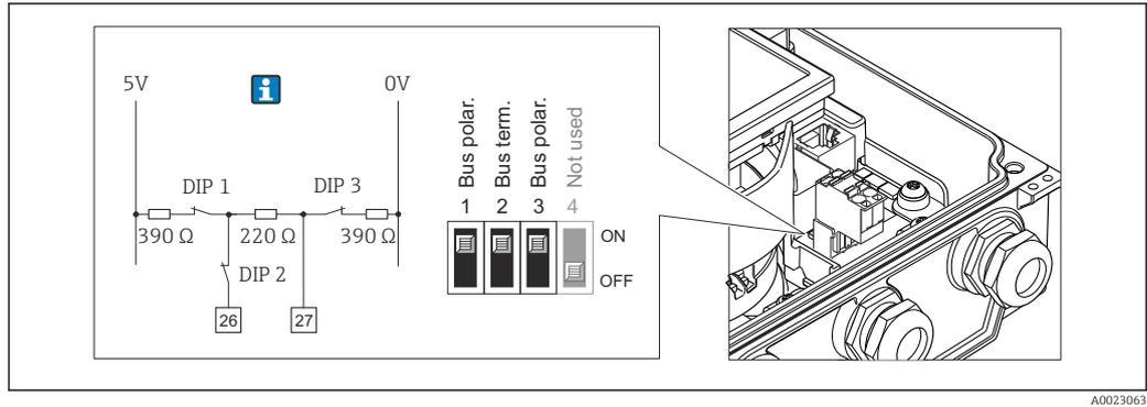
18 Termination using DIP switches on the I/O electronics module (for baud rates < 1.5 MBaud)
