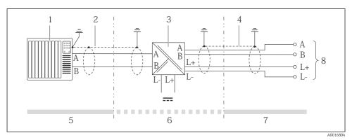
14 Electrical connection between the transmitter and Safety Barrier Promass 100
