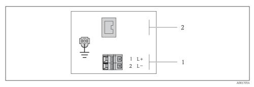
EtherNet/IP terminal assignment
