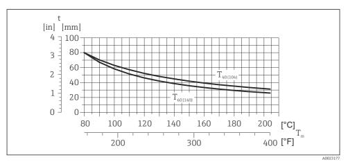
If a Maximum recommended insulation thickness depending on the temperature of the medium and the ambient temperature
