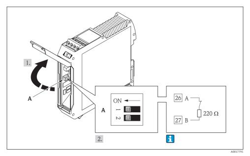
Ita Terminating resistor can be enabled via DIP switch in the Safety Barrier Promass 100
