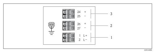
6 Terminal assignment 4-20 mA HART with pulse/frequency/switch output
