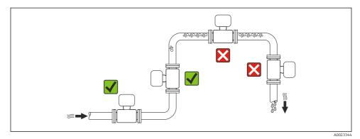
Installation in down pipes
