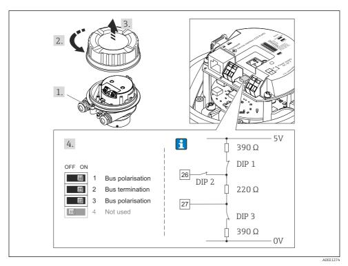
■ 16 Termination using DIP switches on the I/O electronics module (for baud rates < 1.5 MBaud)
