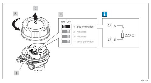
I7 Terminating resistor can be enabled via DIP switch on the main electronics module
