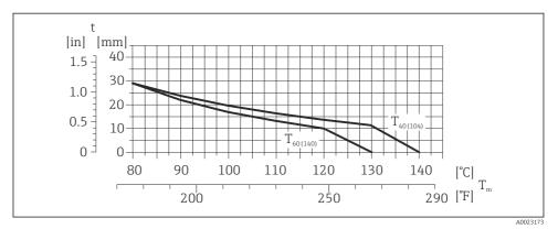
Image: 3 Maximum recommended insulation thickness depending on the temperature of the medium and the ambient temperature
