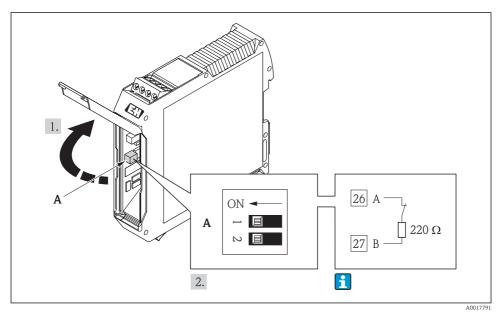
■ 9 Terminating resistor can be enabled via DIP switch in the Safety Barrier Promass 100
