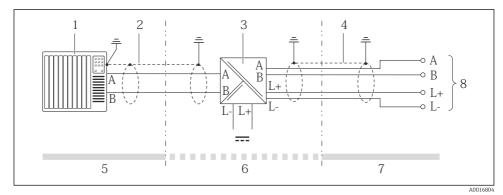
■ 8 Electrical connection between the transmitter and Safety Barrier Promass 100
