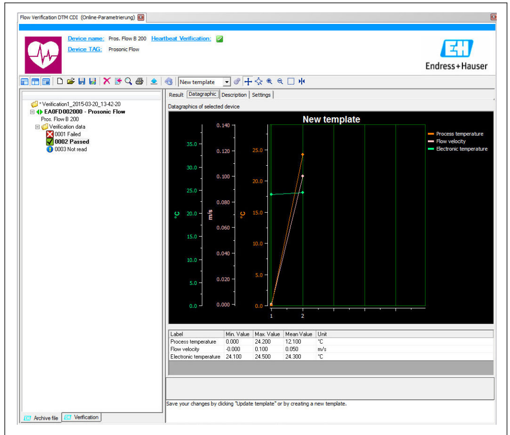
11 "Trend visualization": Template shows the data in chronological order; the data points are referenced by the verification ID (X-axis), the Y-axis is displayed as defined in the configuration
