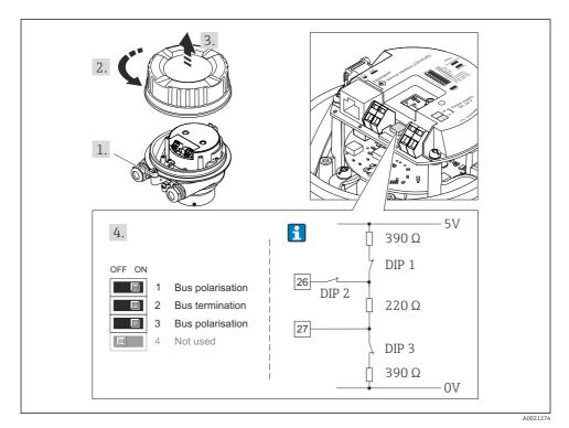
■ 14 Termination using DIP switches on the I/O electronics module (for baud rates < 1.5 MBaud)
