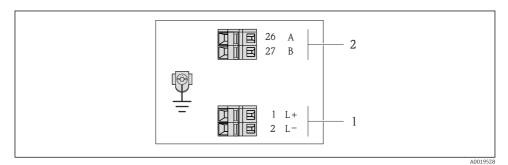
6 Modbus RS485 terminal assignment, connection version for use in non-hazardous areas and Zone 2/Div. 2
