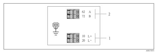
Image: 7 Modbus RS485 terminal assignment, connection version for use in intrinsically safe areas (connection via Safety Barrier Promass 100)
