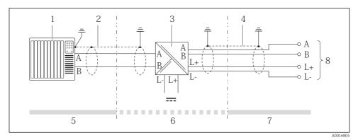
Electrical connection between the transmitter and Safety Barrier Promass 100
