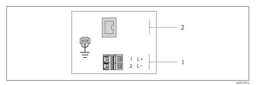
*EtherNet/IP terminal assignment*
