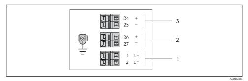
4 Terminal assignment 4-20 mA HART with pulse/frequency/switch output
