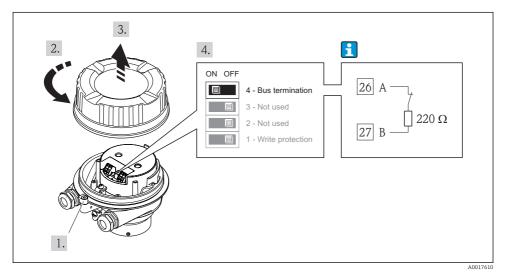
15 Terminating resistor can be enabled via DIP switch on the main electronics module
