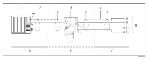
Electrical connection between the transmitter and Safety Barrier Promass 100
