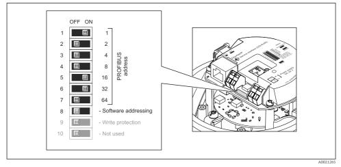
■ 13 Addressing using DIP switches on the I/O electronics module
