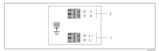
7 Modbus RS485 terminal assignment, connection version for use in intrinsically safe areas (connection via Safety Barrier Promass 100)
