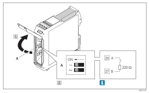
■ 16 Terminating resistor can be enabled via DIP switch in the Safety Barrier Promass 100
