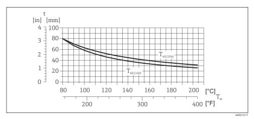
Image: 3 Maximum recommended insulation thickness depending on the temperature of the medium and the ambient temperature
