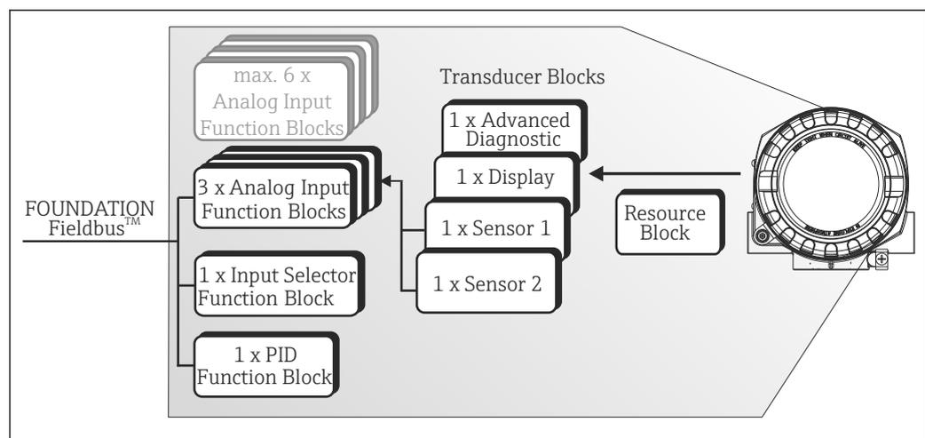
19 Block model of the temperature field transmitter
