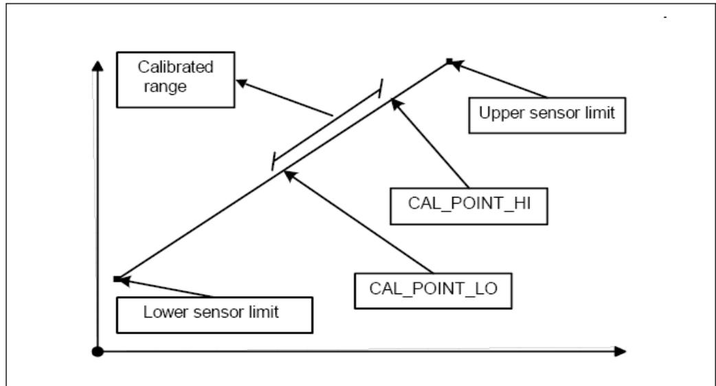
21 Linear scaling of temperature-linear curve
