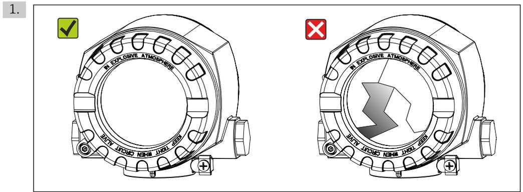
Unpack the temperature transmitter carefully. Is the packaging or content damaged?
