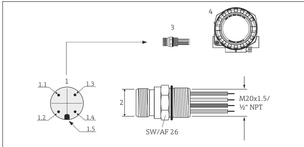
7 Connectors for connecting to the FOUNDATION Fieldbus
