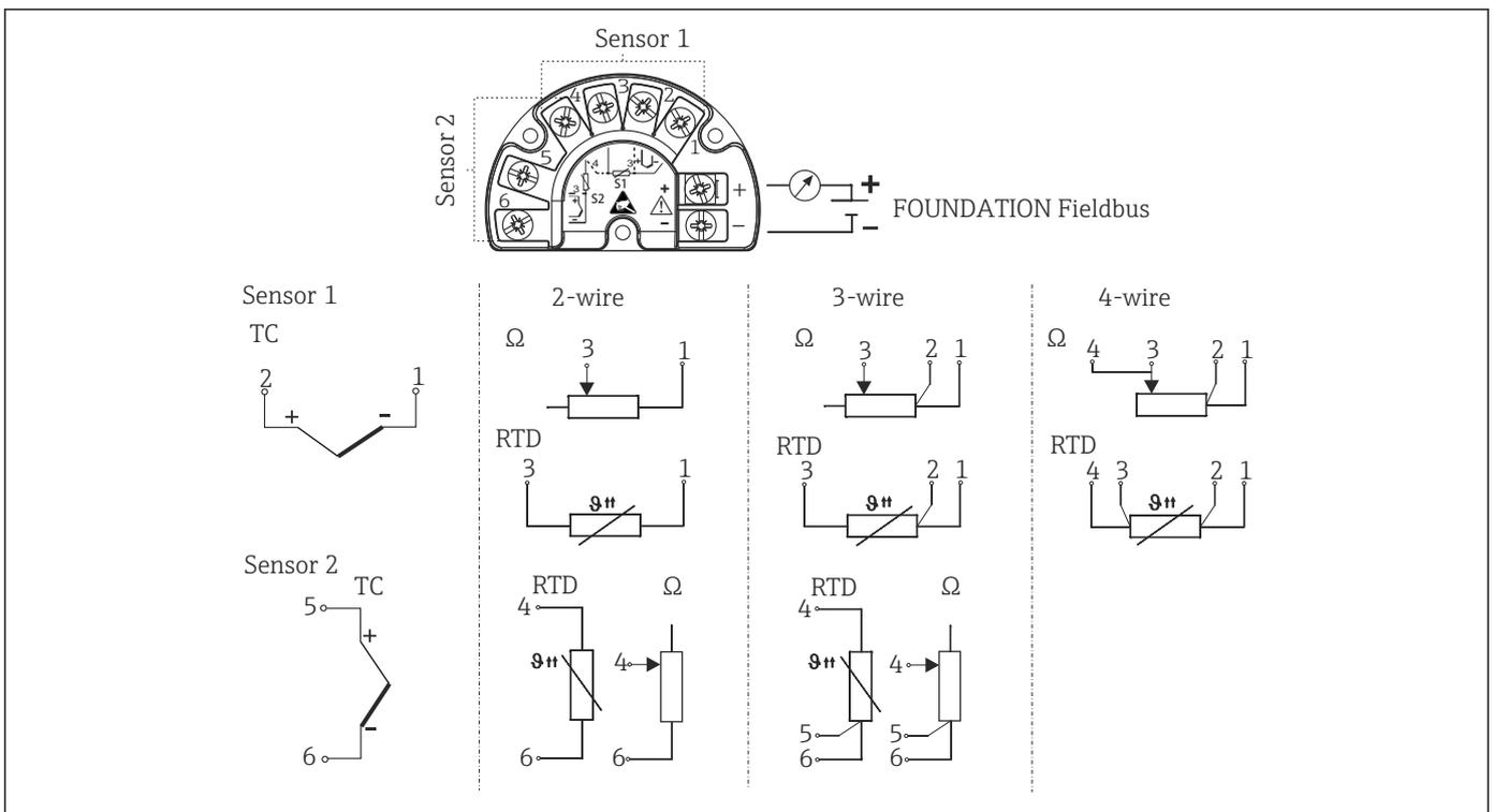
5 Wiring the field transmitter
