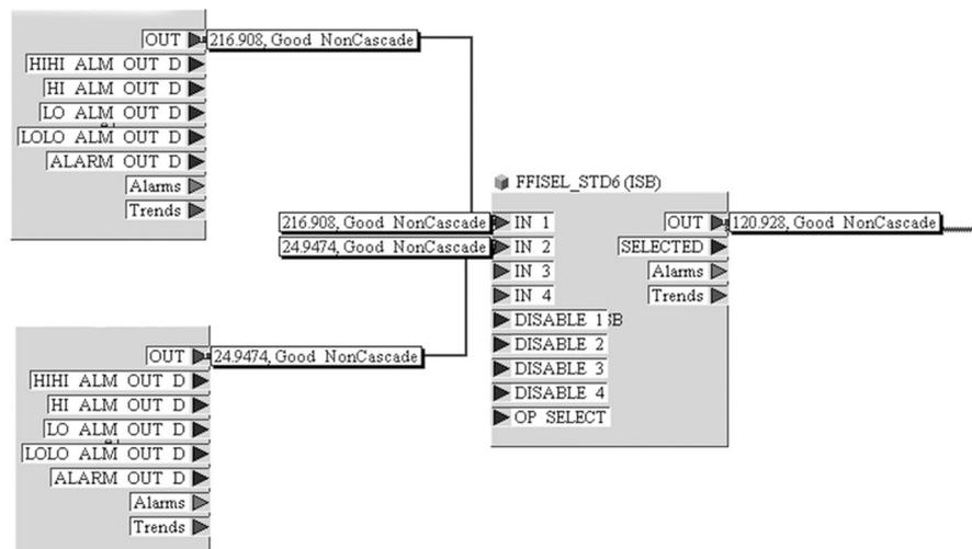
15 Connecting function blocks with the aid of the “NI-FBUS Configurator”. Example: Averaging (output OUT in the Input Selector Block) of two temperature inputs (OUT in the Analog Input Blocks 1 and 2).
