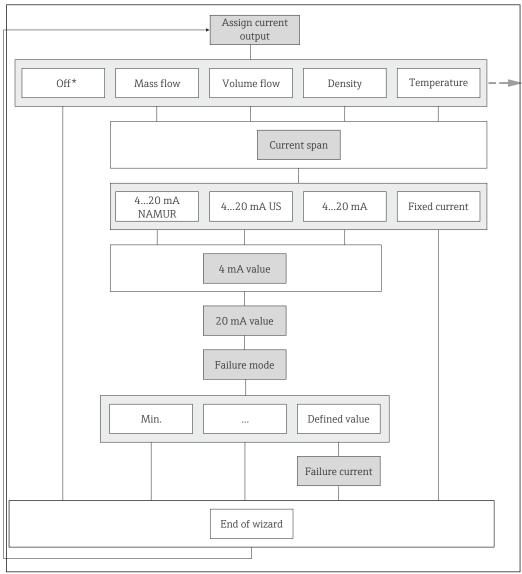
"Current output 1 to 2" wizard in the "Setup" menu (part 1) *Off\** = *Option only for current output 2*
