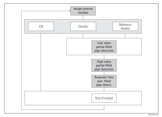
■ 27 "Partially filled pipe detection" wizard in the "Setup" menu
