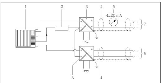
Connection example for HART input with a common negative
