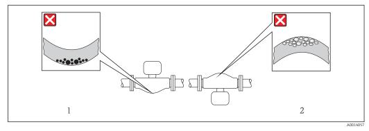
■ 5 Orientation of sensor with curved measuring tube
