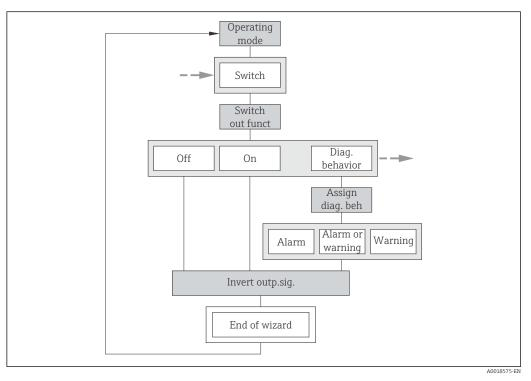
$\blacksquare$  22 "Pulse/frequency/switch output" wizard in the "Setup" menu: "Operating mode" parameter "Switch" option (part 1)
