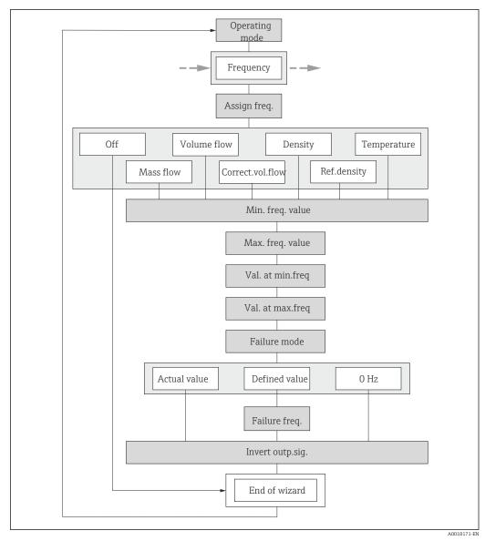
$\blacksquare~21~$  "Pulse/frequency/switch output" wizard in the "Setup" menu: "Operating mode" parameter"Frequency" option
