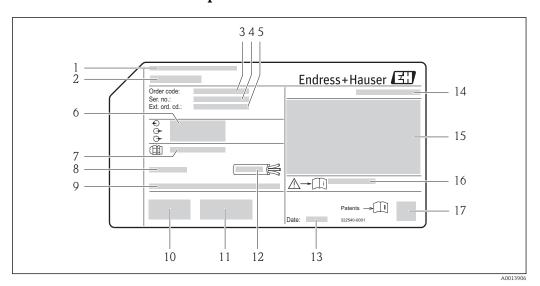
■ 2 Example of a transmitter nameplate
