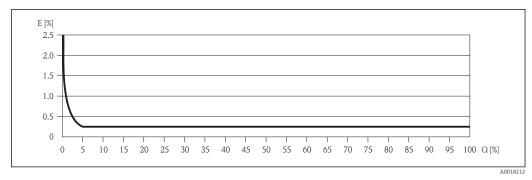
■ 36 Maximum measured error in % o.r. (example: DN 25)
