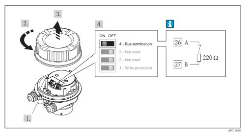
I2 Terminating resistor can be enabled via DIP switch on the main electronics module
