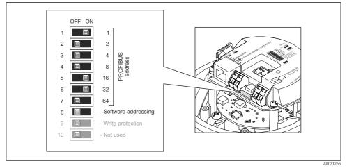
■ 10 Addressing using DIP switches on the I/O electronics module
