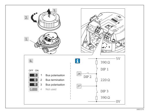
■ 11 Termination using DIP switches on the I/O electronics module (for baud rates < 1.5 MBaud)</p>
