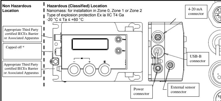
Notes: : Intrinsically safe installation for type of explosion protection Ex ia IIC T4.
